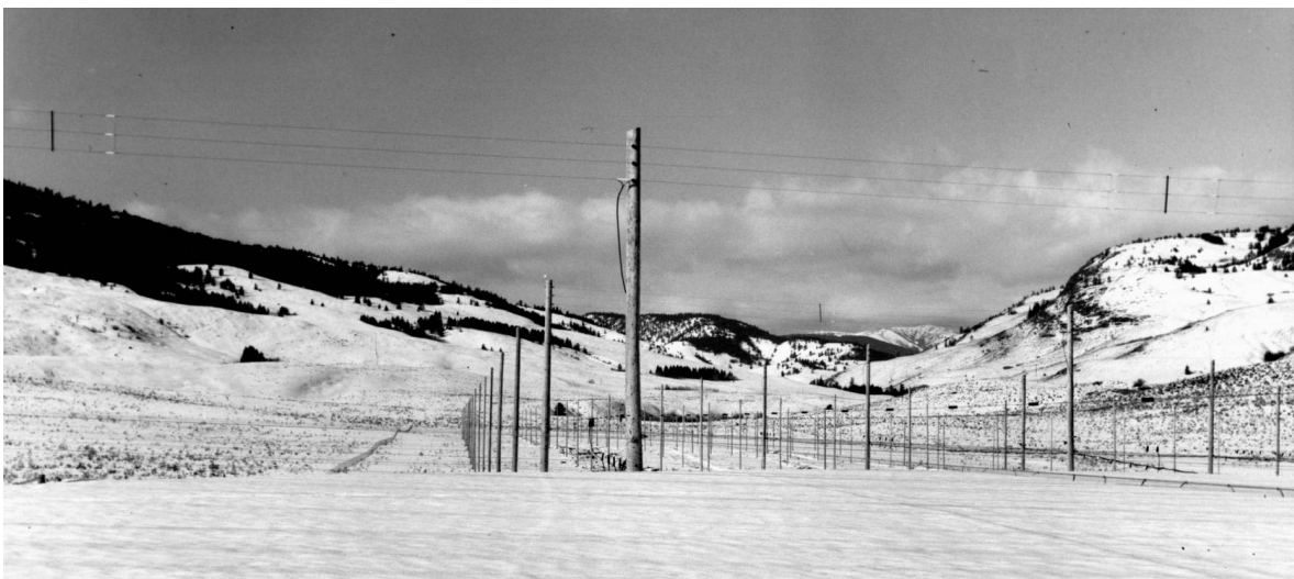
Dipoles at the East end of the 10-MHz array's East-West arm (Dominion Observatory photo)
