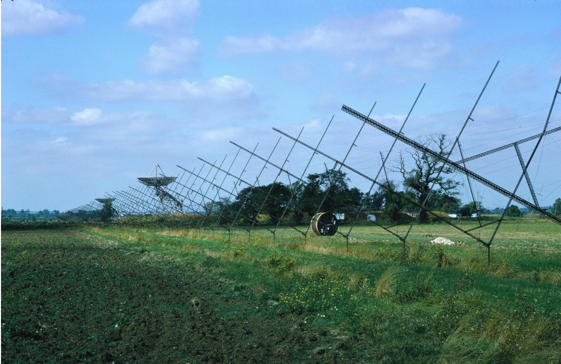
The 3300-ft East-West arm of the 38-MHz aperture synthesis telescope built by Carman Costain at Lord's Bridge (Photo credit - Alan Bridle)
