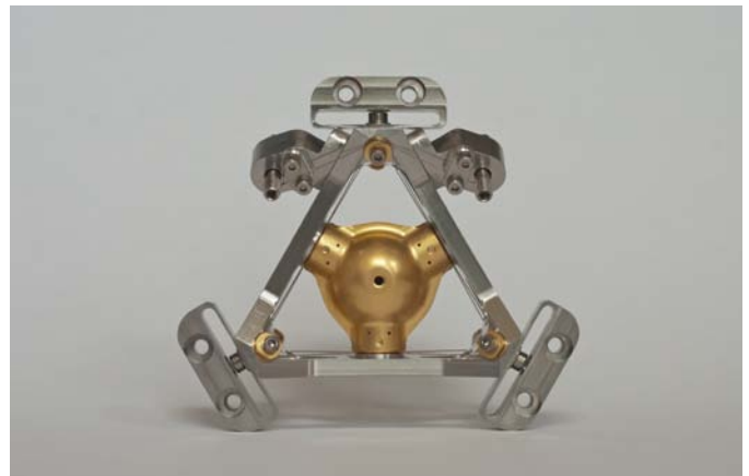
Fig. 6 Prototype of the hot source and suspension.
